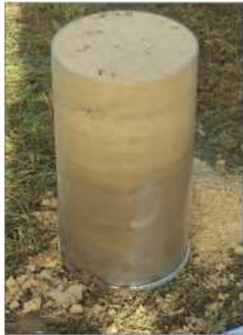
Layered soil in a PMMA cartridge
