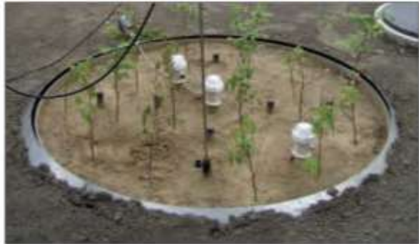
Root studying with rhizotrons and microcameras
