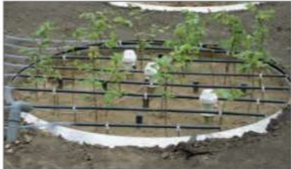
Lysimeter with irrigation system and young beeches
