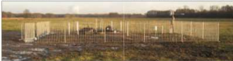
Completed lysimeter station including a weather station
