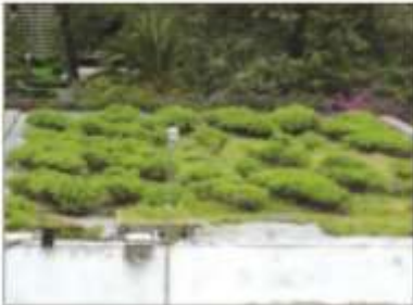
Measuring plots with weighing lysimeters and vegetation
