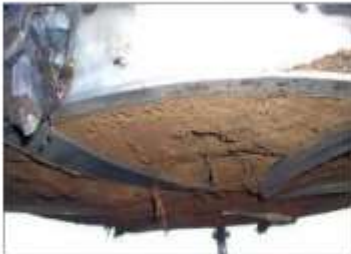
Base cutting with steel fins of a 0.5 m³ soil monolith
