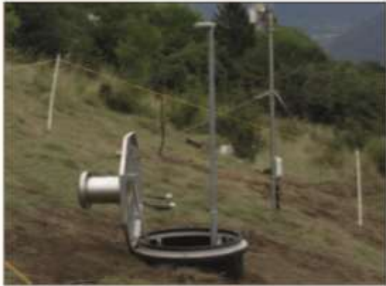
Access shaft of the lysimeter station
