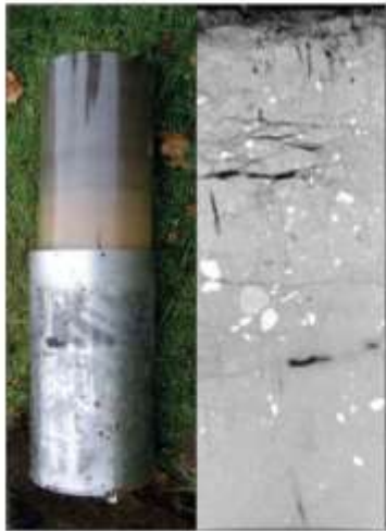
PMMA cartridges make the soil column and its layers visible additionally computer tomography enables to even look inside the soil column to find cracks or roots
