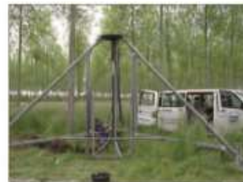
Cutting of a 1 m 2 soil monolith
