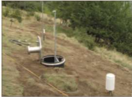
Hillside lysimeter at Sierre/Switzerland direct after installation
