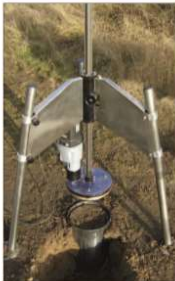
Cutting of a 0,03 m 2 (ø 20 cm) laboratory soil column
