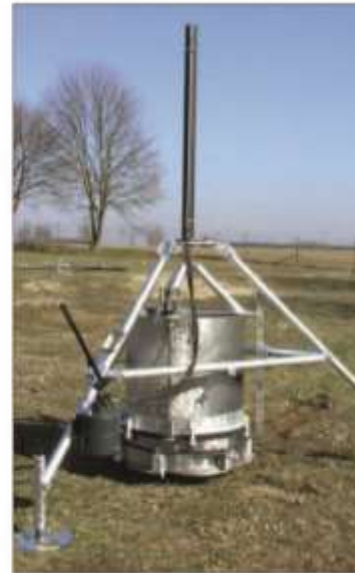
Excavation technology for a 0,5 m 2 soil monolith
