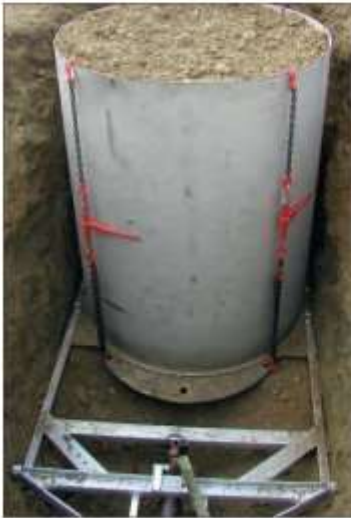
Base cutting with a cut-off plate of a 2 m³ soil monolith
