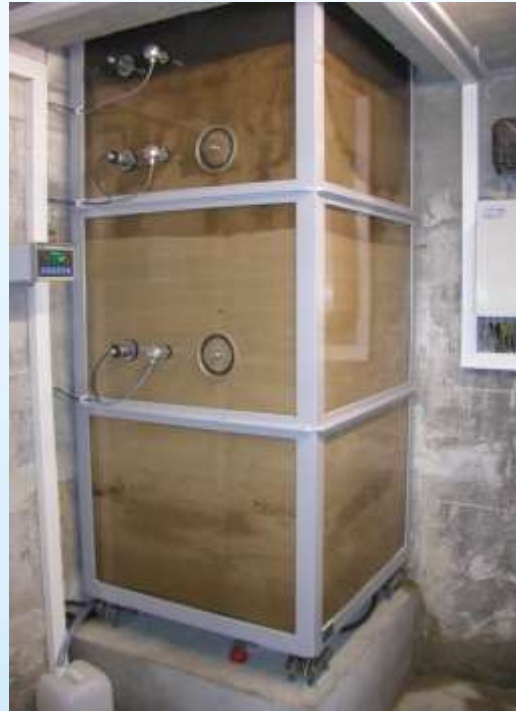
10 weighable lysimeter for non-invasive root observation, and the detection of water and solute fluxes
