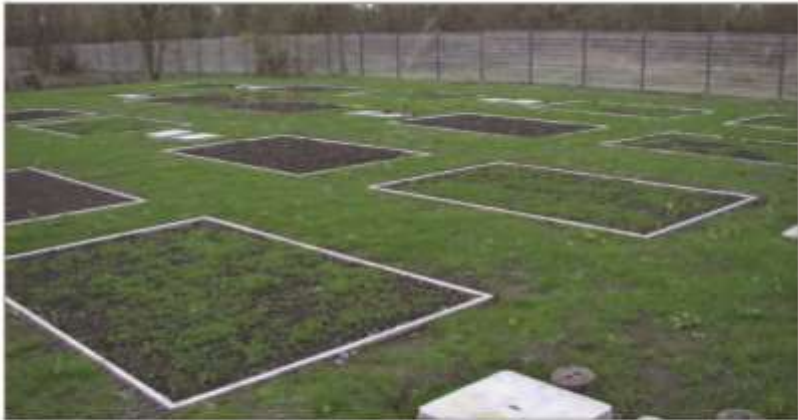
Photolysimeter with different vegetation the data loggers are stored weatherproof in the grey boxes
