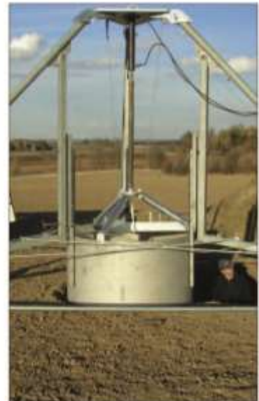
Excavation technology for a 2 m 2 soil monolith
