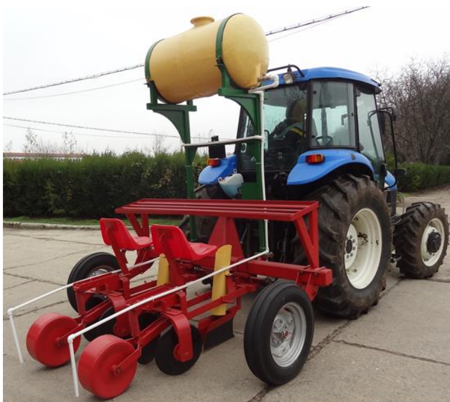
Model experimental de echipament tehnic de plantat tuberculi topinambur
